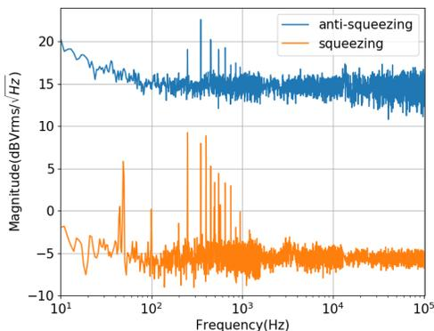
FIG. 3. Squeezing spectrum with frequency below 50Hz contaminated by back-scattering and beam pointing noise
