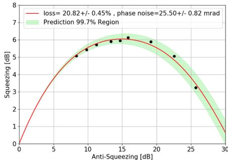
FIG. 2. We measured squeezing and anti-squeezing level with pump power from 20mW to 60mW with an interval of 5mW. These points are fit with equation 2 to give us loss of 20.82 percent and phase noise of 25.5mrad
