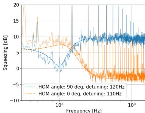
FIG. 4. Frequency dependent squeezing with detuning around 100Hz. Comparing this with figure 3, we can see the effect of filter cavity
